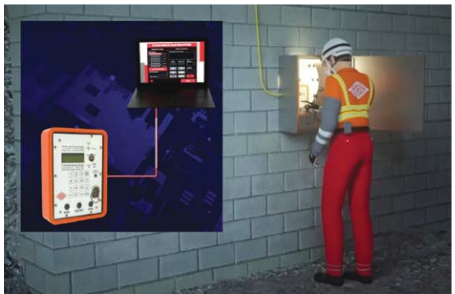
With centralized blasting equipment, such as E*STAR CUBE from Austin Powder, operators can now initiate multiple blasts from the surface with zero personnel in the mine. (Image: Austin Powder)
