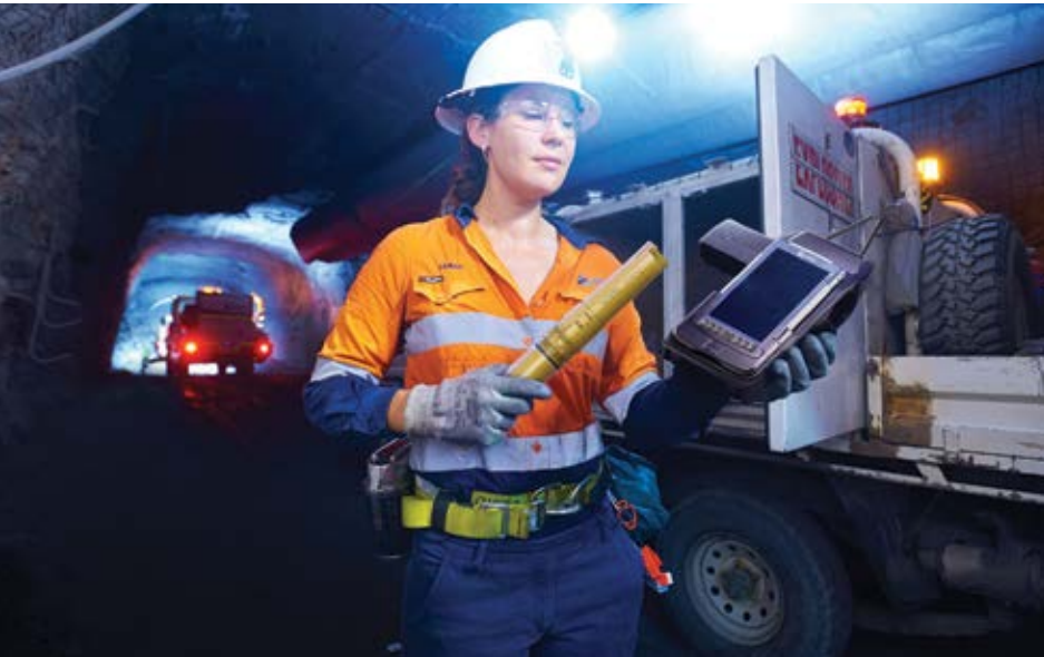
Orica's WebGen 200 Underground Pro wireless initiating system removes personnel from harm's way during blasting. (Photo: Orica)
