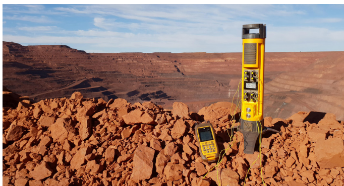
Figure 5. Electronic initiation systems allow for enhanced timing accuracy and precise blast designs.
