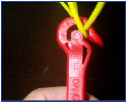
Figure 86 - Shock tube crossed over in the connector block.
