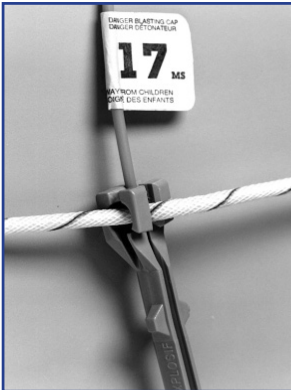
Figure 107 - J-Hook improperly connected to the trunkline
