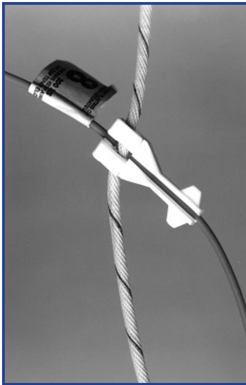
Figure 105 - Shock tube should leave J-Hook in a straight line. The above image shows an "Angle Cut-off".
