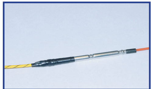
Figure 79 - End priming. The detonator is securely taped to the end of the detonating cord.
