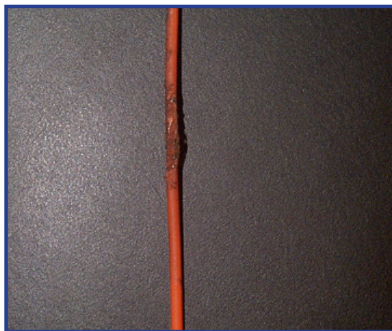
Figure 113 - Shock tube damaged by cord tail. The shock tube can also be severed.
