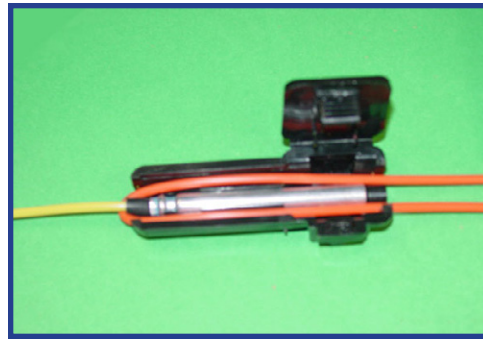
Figure 59 - Shot initiation using NONEL Starter unit. Note shock tube lead position so it will be initiated in both directions.
