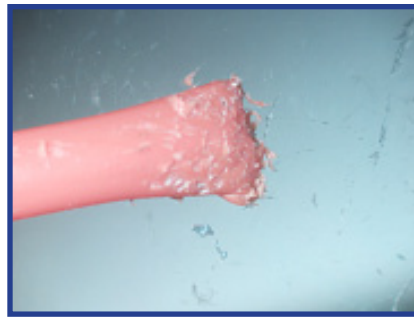
Figure 129 & 130 - Shock tube that has been cut by a pinch-smash break.
