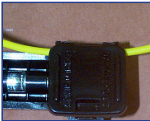
Figure 101 - Shock tube shut in Bunch Block hinge. Misfire may occur.
