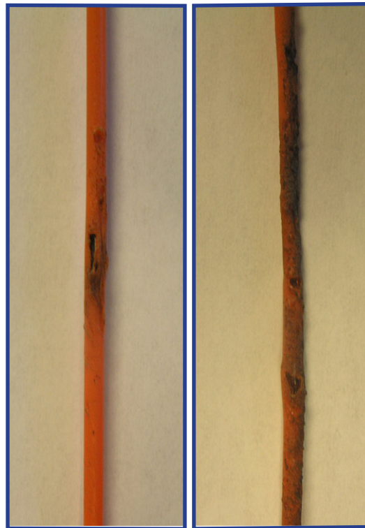
Figure 104 - Left shock tube damaged by detonating cord as shown in Figure 111. Right shock tube damage is due to extended linear contact with detonating cord.
