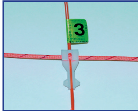
Figure 34 - Correct J-Hook connection.
