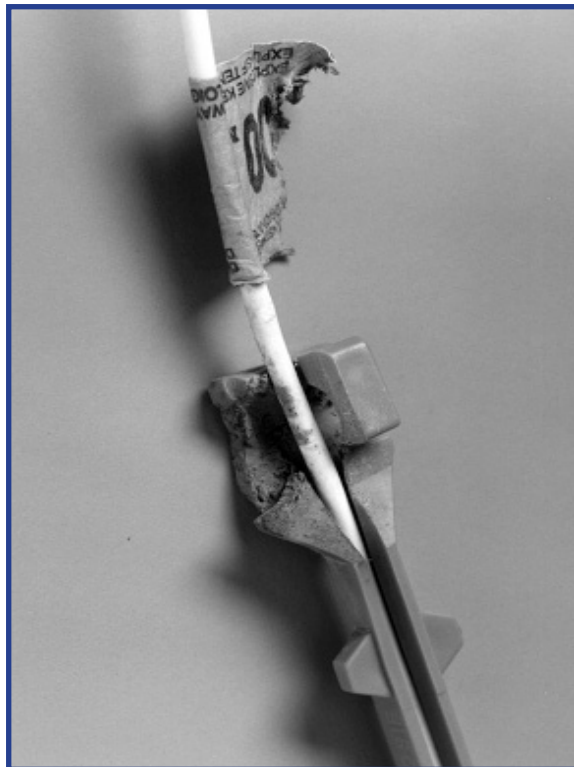
Figure 108 - Result of the hook-up at left; can result in an initiation failure
