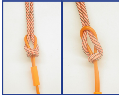
Figure 76 - Front (left) and back (right) views of double-wrap square knot connecting SL unit and PRIMACORD 3.
