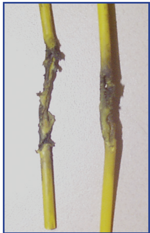
Figure 102 - Shock tube on the left failed to initiate because it was positioned between the Bunch Block lid and hinge. (unit returned from customer)
