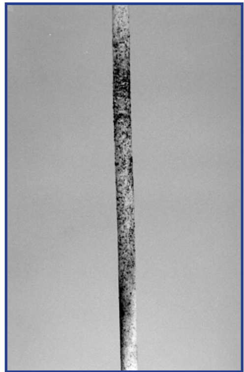
Figure 106 - Shock tube damaged by detonating cord
