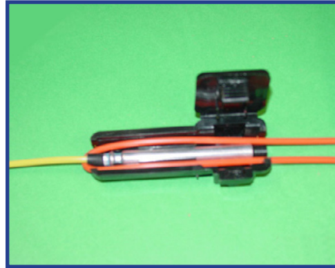
Figure 81 - Initiation using a Bunch Block.
