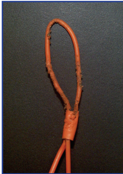
Figure 111 - Result of bad knot.
