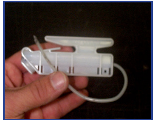
Figures 123 & 124 - Failures may result if shock tube contacts cord.
