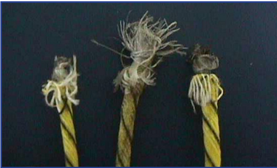
Figure 125 - Center cord was returned by a customer and shows the typical signs associated with an “Angle” or “Cross Talk” cut-off.
