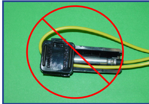
Figure 60 - Incorrect hook-up; shock tube lead is bent around the nose of the Bunch Block.
