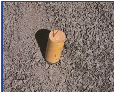
Figure 134 - Primer assembly with shock tube lead broken due to pinch smash.
