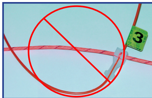
Figure 31 - Incorrect connection of J-Hook to trunkline; shock tube lead crosses over trunkline. Cut-offs or misfires may result.
