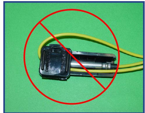
Figure 11 - Shock tube bent around nose of Bunch Block. Cut-off may result.
