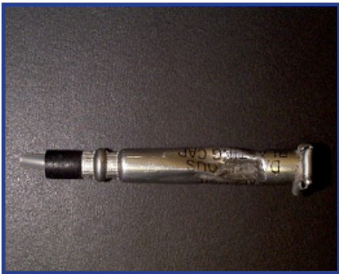
Figure 119 - Detonator after functioning with detonating cord NOT in groove of the connector.
