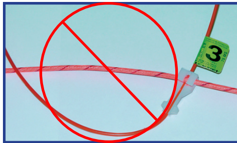
Figure 35 - Incorrect J-hook connection. Crossover may cause cut-offs or misfires.
