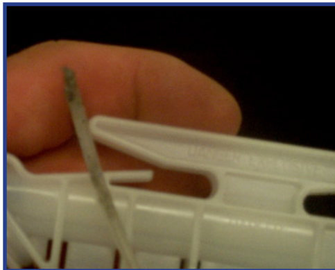
Figures 123 & 124 - Failures may result if shock tube contacts cord.
