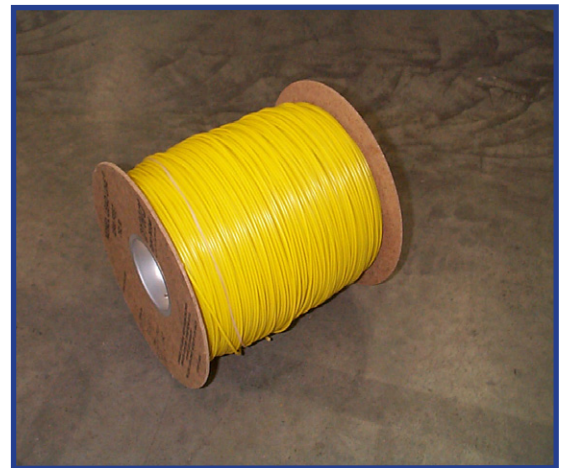
Figure 142 - Incorrect orientation for transportation. Powder migration may occur.
