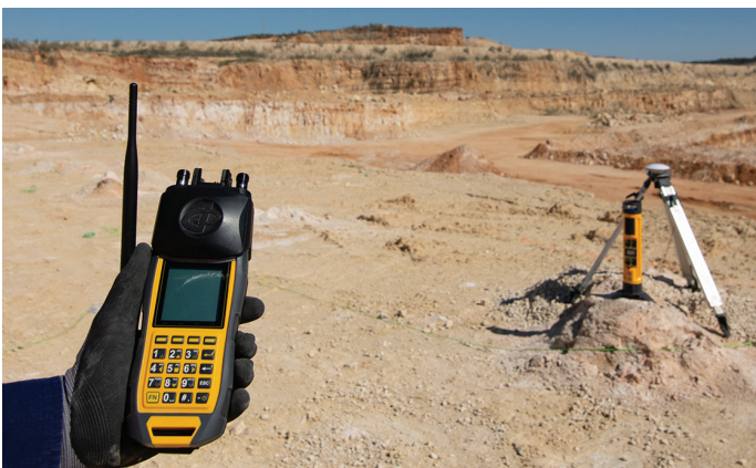
Easily setting up the DGPS base.
